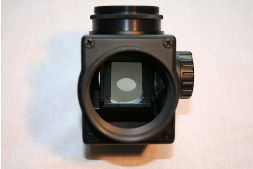
Fig. 18.4 Beamsplitter in place
